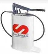
Maximum pressure range between 175 to 350 bar (2,500 to 5,000 psi) with a delivery of 20 g, 15 g or 10 g per stroke depending on the position of the lever chosen. Ideal pump for high pressure greasing and valve flushing. Includes 1,5 m high pressure hose with a three-jaw hydraulic
