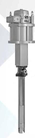
Ultra-High pressure pumps designed for grease injection in wireline pressure control equipment. Can also be used for wellhead sealant injection for valve integrity services.
